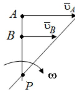
$$\begin{aligned} \vec{v}_A &\parallel \vec{v}_B \\ \vec{v}_A &\perp AB; \end{aligned}$$
