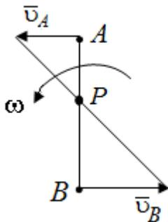
$$\begin{aligned} \vec{v}_A &\perp AB; \\ \vec{v}_A &\parallel \vec{v}_B \end{aligned}$$
