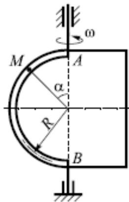
$$\omega = 6t - 2t^2 \text{ c}^{-1}; \quad v_{\text{отн}} = 5\pi t^2 \frac{\text{см}}{\text{с}}; \\ t = 1 \text{ с}; \quad R = 5 \text{ см}; \quad \alpha = 45^\circ$$
