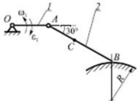
$$\omega_1 = 3 \frac{\text{рад}}{\text{с}}; \quad \varepsilon_1 = 6 \frac{\text{рад}}{\text{с}^2}; \quad OA = 15 \text{ см}; \\ AB = 25 \text{ см}; \quad BC = 15 \text{ см}; \quad R = 20 \text{ см}$$
