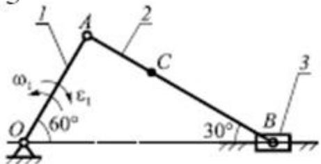
$$\omega_1 = 1 \frac{\text{рад}}{\text{с}}; \quad \varepsilon_1 = 3 \frac{\text{рад}}{\text{с}^2}; \quad OA = 20 \text{ см}; \\ AC = 12 \text{ см}$$
