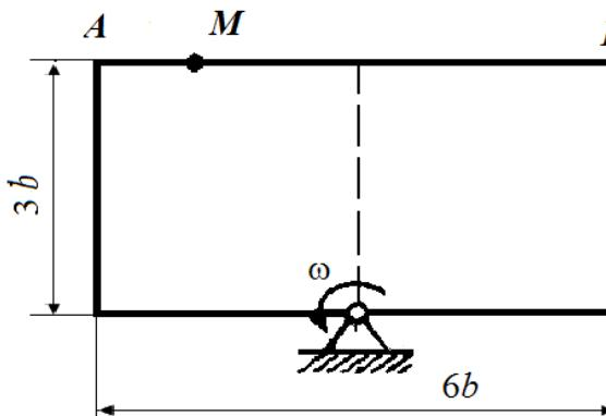
$\omega = 3 \text{ c}^{-1}$<br>$S = 80(2t^2 - t^3) - 48, \text{ см}$<br>$t = 1 \text{ с}; b = 8 \text{ см}$                                                            |
