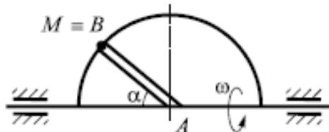
$$\omega = 2t - 4t^2 \text{ c}^{-1}; V_{\text{отн}} = 36 \sin \frac{\pi t}{3} \frac{\text{см}}{\text{с}}$$
