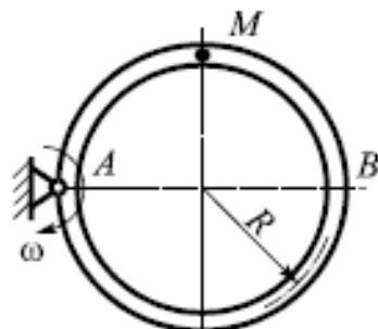
$$\omega = 7t^2 - 3 \text{ c}^{-1}; \quad v_{\text{отн}} = 40t^2 \frac{\text{см}}{\text{с}}; \\ t = 1 \text{ с}; \quad R = 6 \text{ см}$$
