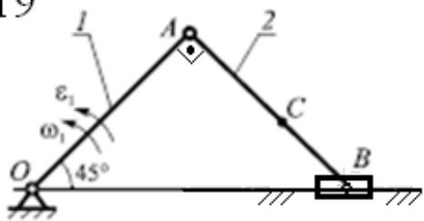
$$\omega_1 = 3 \frac{\text{рад}}{\text{с}}; \quad \varepsilon_1 = 4 \frac{\text{рад}}{\text{с}^2}; \quad OA = 20 \text{ см}; \\ BC = 8 \text{ см};$$
