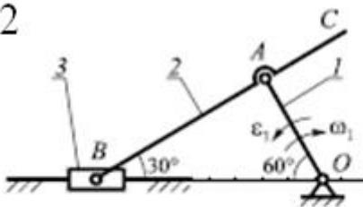
$$\omega_1 = 1 \frac{\text{рад}}{\text{с}}; \quad \varepsilon_1 = 4 \frac{\text{рад}}{\text{с}^2}; \quad AB = 30 \text{ см}; \\ BC = 45 \text{ см}$$
