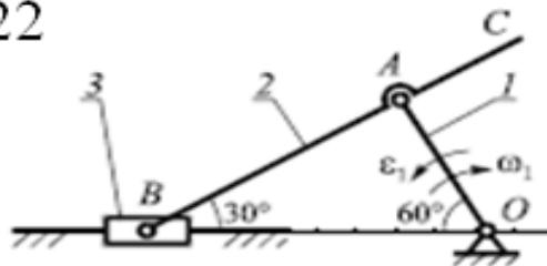
$$\omega_1 = 1 \frac{\text{рад}}{\text{с}}; \quad \varepsilon_1 = 4 \frac{\text{рад}}{\text{с}^2}; \quad AB = 30 \text{ см}; \\ BC = 45 \text{ см}$$
