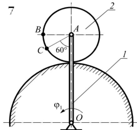
$$\varphi_1 = 8t - 2t^2 \text{ rad}; \quad t = 1 \text{ с}; \\ OA = 50 \text{ см}; \quad AB = 15 \text{ см}$$
