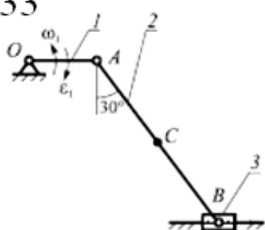
$$\omega_1 = 4 \frac{\text{рад}}{\text{с}}; \quad \varepsilon_1 = 6 \frac{\text{рад}}{\text{с}^2}; \quad OA = 10 \text{ см}; \\ AB = 30 \text{ см}; \quad BC = 15 \text{ см}$$
