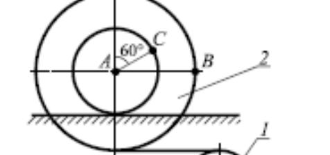
$\omega_1 = 3t^2 \text{ рад}$<br>$t = 2 \text{ с}$<br>$r = 20 \text{ см}$ ; $AB = 40 \text{ см}$ ; $AC = 25 \text{ см}$                                                             |
