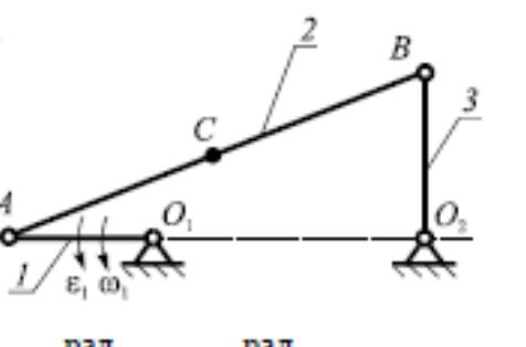
$\omega_1 = 3 \frac{\text{рад}}{\text{с}}$ ; $\epsilon_1 = 7 \frac{\text{рад}}{\text{с}^2}$ ; $O_1A = 15 \text{ см}$<br>$O_2B = 20 \text{ см}$ ; $O_2A = 40 \text{ см}$ ; $AC = BC$ |
