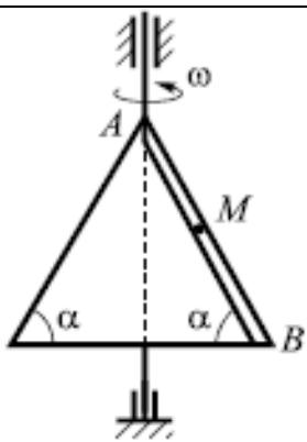
$$\omega = 5t - t^2 \text{ c}^{-1}; \quad v_{\text{отн}} = 4t^2 + 2 \frac{\text{см}}{\text{с}}; \\ t = 1 \text{ с}; \quad AM = 4 \text{ см}; \quad \alpha = 60^\circ$$
