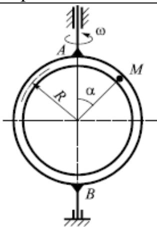
$$\omega = 2 \sin \frac{\pi t}{3} \text{ c}^{-1}; \quad v_{\text{отн}} = 4\pi t^2 \frac{\text{см}}{\text{с}}; \\ t = 1 \text{ с}; \quad R = 4 \text{ см}; \quad \alpha = 45^\circ$$
