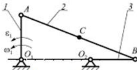
$$\omega_1 = 1 \frac{\text{рад}}{\text{с}}; \quad \varepsilon_1 = 1 \frac{\text{рад}}{\text{с}^2}; \quad AB = 50 \text{ см}; \\ O_1A = O_2B = 20 \text{ см}; \quad BC = 25 \text{ см}$$
