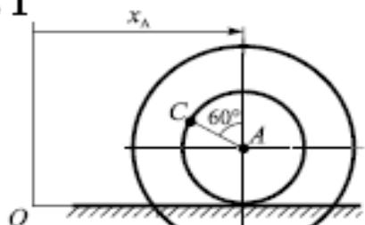
$$x_A = 50t - 10t^2 \text{ см}; \quad t = 1 \text{ с}; \\ AB = 25 \text{ см}; \quad AC = 15 \text{ см}$$
