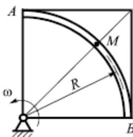
$$\omega = 3t^2 - 2t \text{ c}^{-1}; \quad v_{\text{отн}} = 15t^2 \frac{\text{см}}{\text{с}}; \\ t = 1 \text{ с}; \quad R = 6 \text{ см}$$
