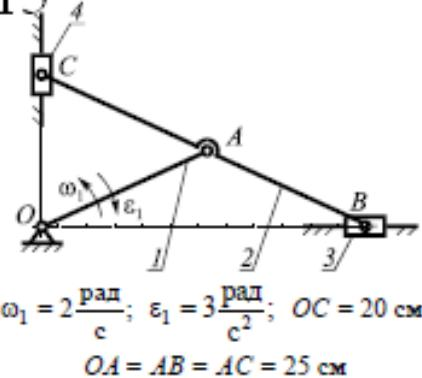
$$\omega_1 = 2 \frac{\text{рад}}{\text{с}}; \quad \varepsilon_1 = 3 \frac{\text{рад}}{\text{с}^2}; \quad OC = 20 \text{ см}; \\ OA = AB = AC = 25 \text{ см}$$
