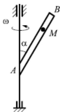
$$\omega = 4 \cos \frac{\pi t}{3} \text{ c}^{-1}; \quad v_{\text{отн}} = 3t^2 - t \frac{\text{см}}{\text{с}}; \\ t = 1 \text{ с}; \quad AM = 6 \text{ см}; \quad \alpha = 30^\circ$$
