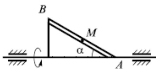
$$\omega = 6t + t^2 \text{ c}^{-1}; v_{\text{отн}} = 50 \sin \frac{\pi t}{4} \frac{\text{см}}{\text{с}};$$
