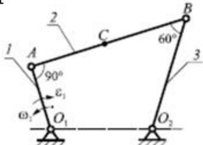
$$\omega_1 = 1 \frac{\text{рад}}{\text{с}}; \quad \varepsilon_1 = 1 \frac{\text{рад}}{\text{с}^2}; \quad O_1A = 30 \text{ см}; \\ O_2B = 50 \text{ см}; \quad AB = 70 \text{ см}; \quad AC = BC$$
