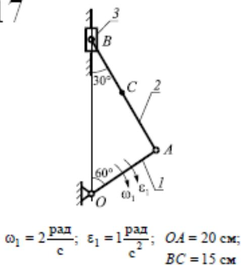
$$\omega_1 = 2 \frac{\text{рад}}{\text{с}}; \quad \varepsilon_1 = 1 \frac{\text{рад}}{\text{с}^2}; \quad OA = 20 \text{ см}; \\ BC = 15 \text{ см}$$
