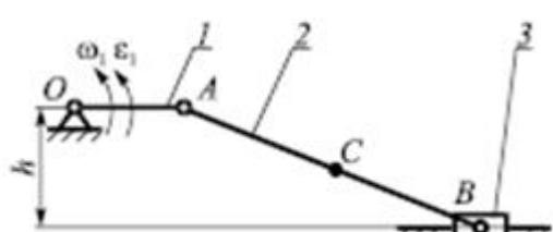
$$\omega_1 = 2 \frac{\text{рад}}{\text{с}}; \quad \varepsilon_1 = 5 \frac{\text{рад}}{\text{с}^2}; \quad OA = 10 \text{ см}; \\ AB = 30 \text{ см}; \quad AC = 15 \text{ см}; \quad h = 12 \text{ см}$$
