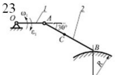
$$\omega_1 = 3 \frac{\text{рад}}{\text{с}}; \quad \varepsilon_1 = 6 \frac{\text{рад}}{\text{с}^2}; \quad OA = 15 \text{ см}; \\ AB = 25 \text{ см}; \quad BC = 15 \text{ см}; \quad R = 20 \text{ см}$$
