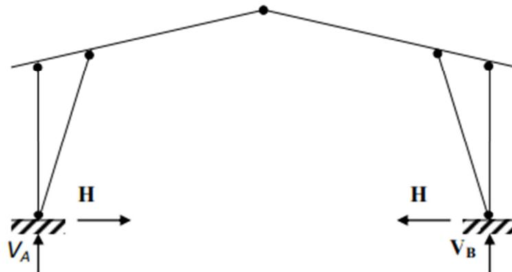
$$H=10\text{кН}; V_b=V_A=20\text{кН}; \alpha=30^\circ.$$
