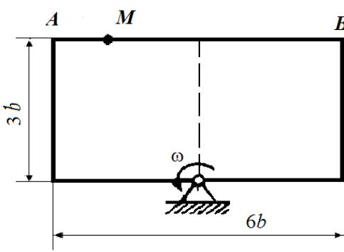
$$\begin{aligned}\omega &= 3 \text{ c}^{-1} \\ S &= 80(2t^2 - t^3) - 48, \text{ см} \\ t &= 1 \text{ с}; \quad b = 8 \text{ см}\end{aligned}$$
