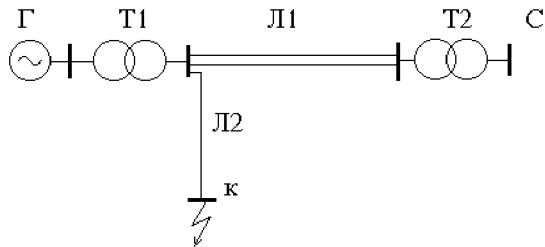
$\Gamma: P = 6 \times 63 \text{ МВт}$  $U = 10.5 \text{ кВ}$  $\cos \varphi = 0.8$  $X_d'' = 0.27$  $L1: l = 27 \text{ км}$  $T1: S = 4 \times 125 \text{ МВА}$  $U = 110/10 \text{ кВ}$  $U_k = 12 \%$  $L2: l = 15 \text{ км}$  $T2: S = 2 \times 250 \text{ МВА}$  $U = 220/110 \text{ кВ}$  $U_k = 9 \%$  $C: U_c = 230 \text{ кВ}$  $S_k'' = 950 \text{ МВА}$  $X_p = 0.4 \text{ Ом/км}$
