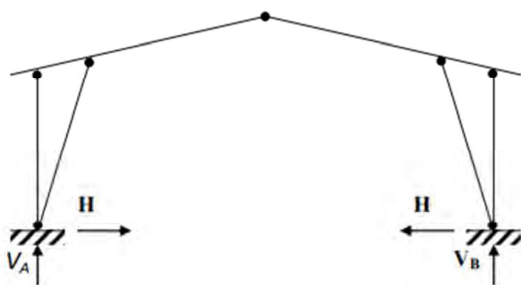
$$H=10 \text{ kN}; V_B=V_A=20 \text{ kN}; \alpha=30^\circ.$$
